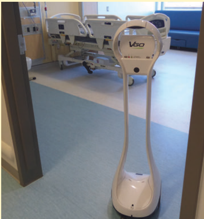
The VGo robot uses a wi-fi connection to allow users to communicate via teleconference as they move from place to place. The robot's screen panel allows the user to see and talk to people who are logged on at another location.
